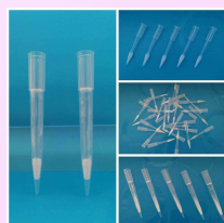
Figure 5. Examples of pipette tips with sorbents
